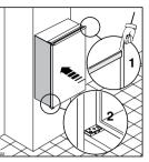
Fit the appliance in the niche by making sure that it stands against the interior surface of the unit on the side where the door hinges of the appliances are fitted. Insert the appliance until the upper strip butts up against the unit (1) and make sure that the lower hinge is in line with the surface of the unit (2).
